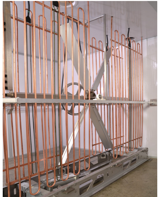
Picture 1: Side view of the heat exchange surface using heat resistance and hot water
