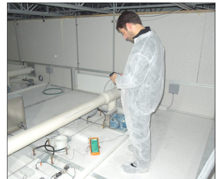
Probes connected to the Resonance device are routed through the incubator roof
