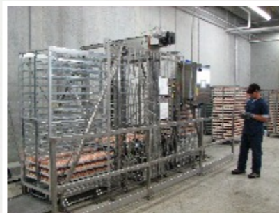
Fully automated system from transport to setter trolley
