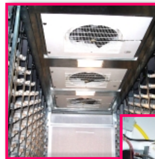
Classic setter with Vostermans plastic fan boards in operational and maintenance positions.
