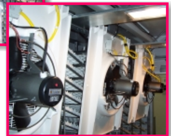
Classic setter with Vostermans plastic fan boards in operational and maintenance positions.
