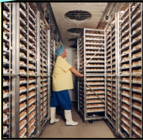
Central access corridor: The Buckeye B16D has a central access corridor that allows easy access for maintenance, cleaning, egg inspection and loading.
