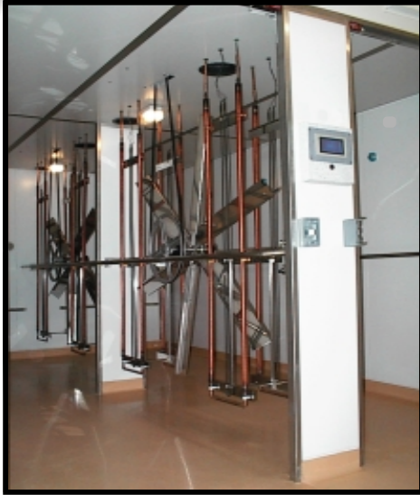
Bio-secure Design: Clear floor area allows the entire machine to be cleaned easily and efficiently after every set.
