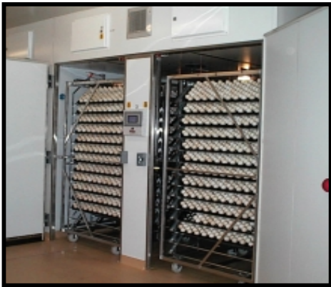
Ultimate ventilation: Avida Single-Stage setters are designed specifically for all-in/all-out duck incubation with one trolley positioned each side of the central fan.
